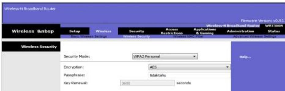
**Gambar 5. Konfigurasi Wireless Security**
