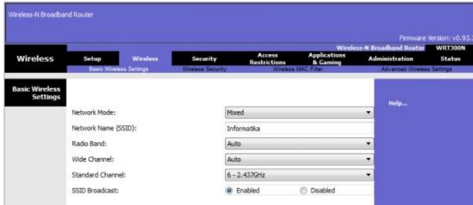
**Gambar 4. Konfigurasi Network Mode, SSID, Channel**
