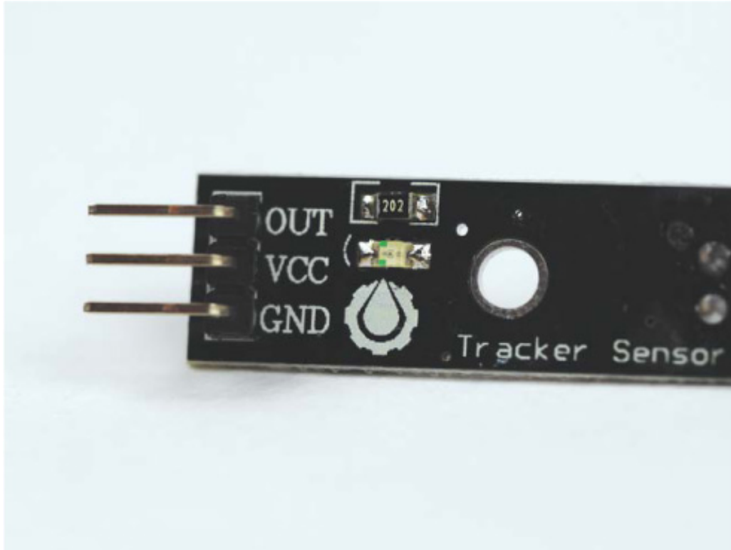
FIGURE 7-10 Pinout of a TCRT5000 IR sensor module
