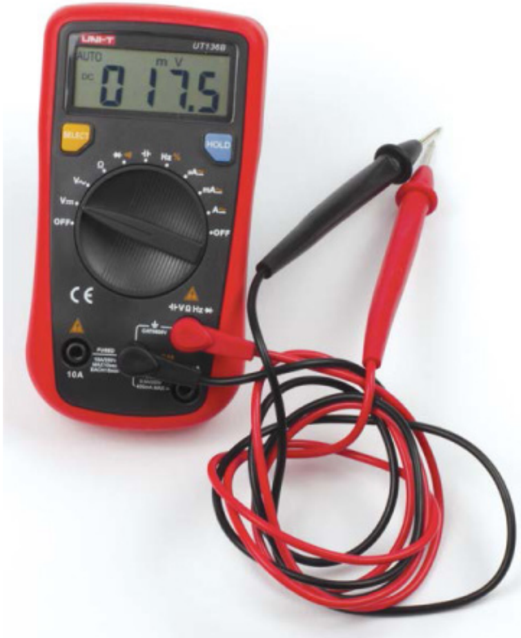
FIGURE 3-17 A multimeter, set to read voltage
