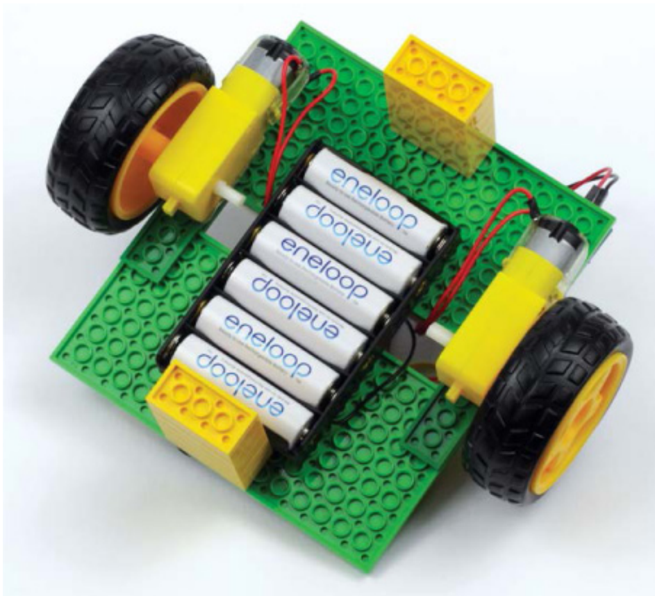
FIGURE 3-15 The underside of the robot with a battery holder attached
