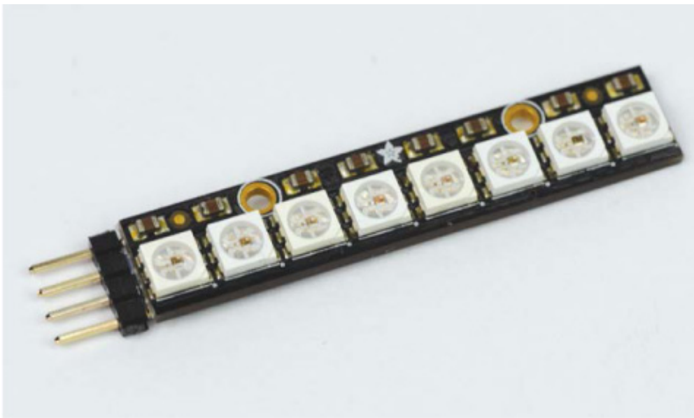
FIGURE 6-4 NeoPixel Stick with headers soldered on
