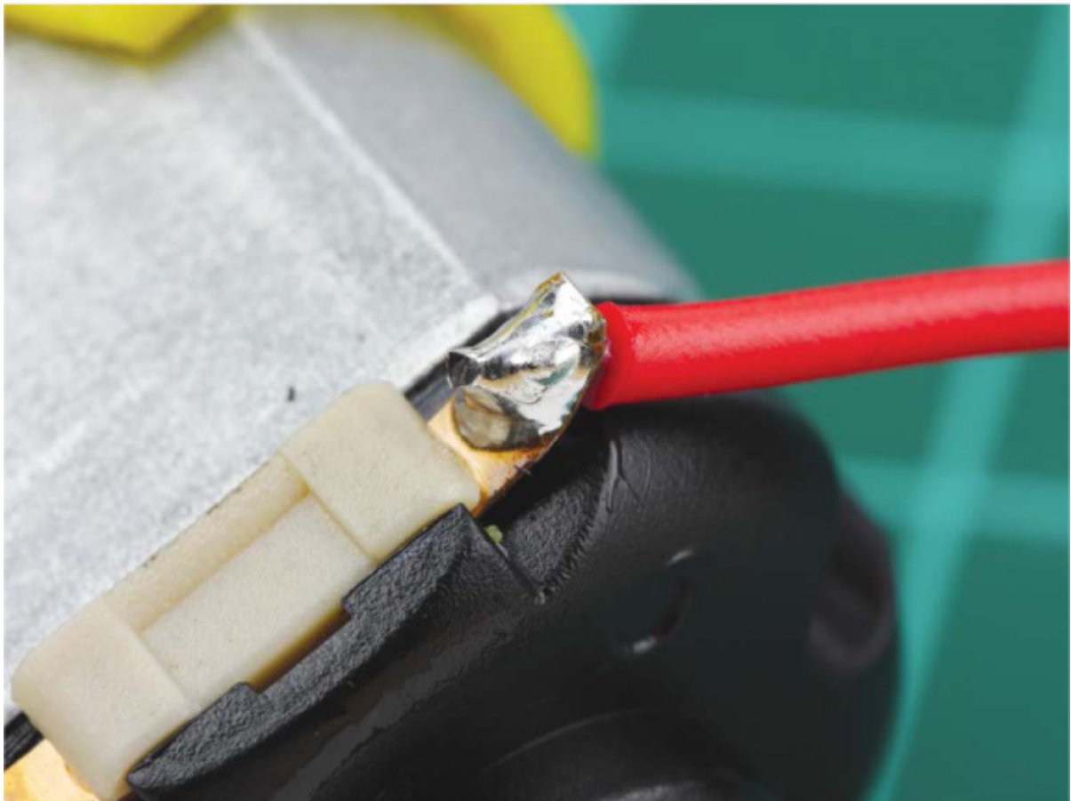
FIGURE D-8 My soldered motor terminal—notice how shiny and cone-shaped the joint is
