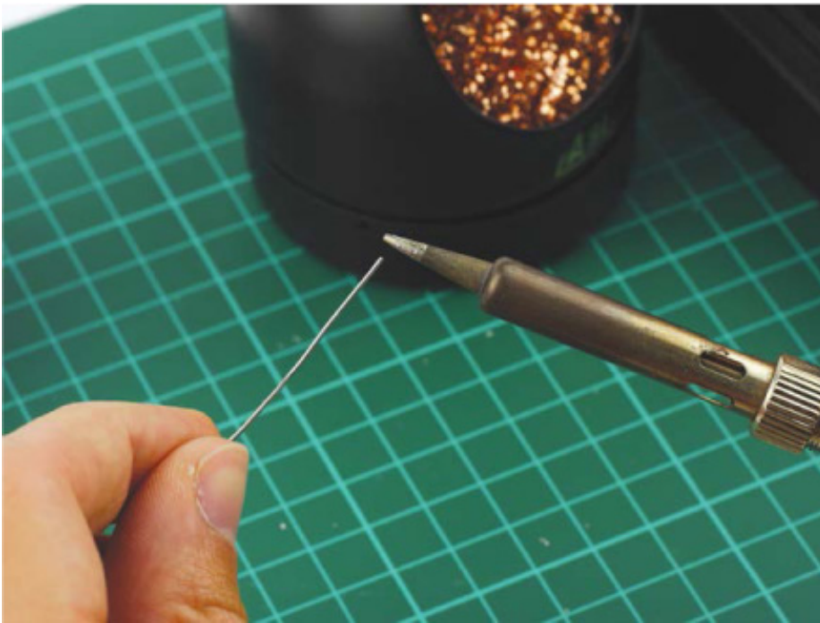
FIGURE D-6 Tinning the tip of my soldering iron
