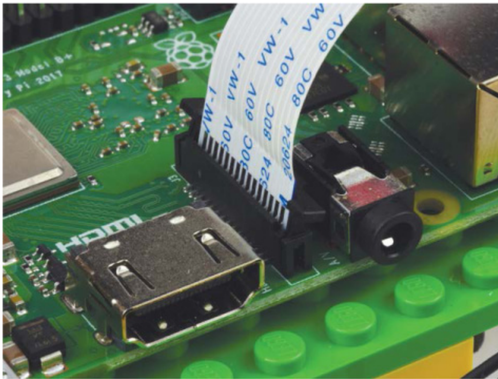
FIGURE 8-5 CSI port with the Camera Module's ribbon cable inserted in the correct direction
