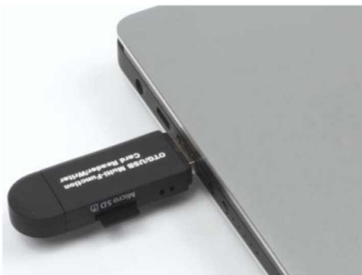
FIGURE 1-7 My USB adapter setup plugged into my laptop, ready for formatting
