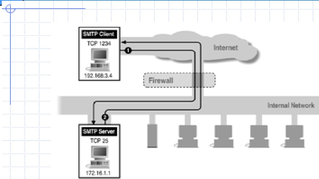
Can block external request to internal server based on port number
