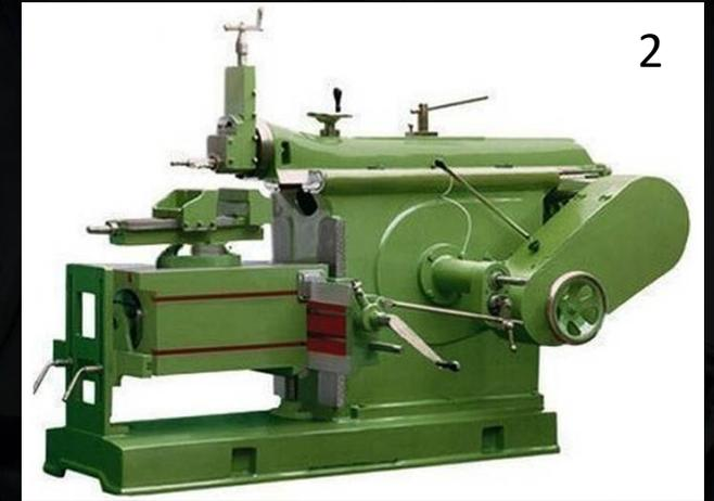
1 Mesin Sekrap Engkol (crank shaper)
