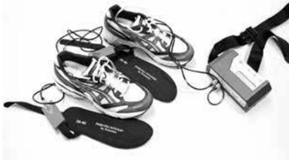
**Figure 16.5** Pressure-measuring insoles are useful tools for measuring pressure on the plantar surface of the feet during gait.
