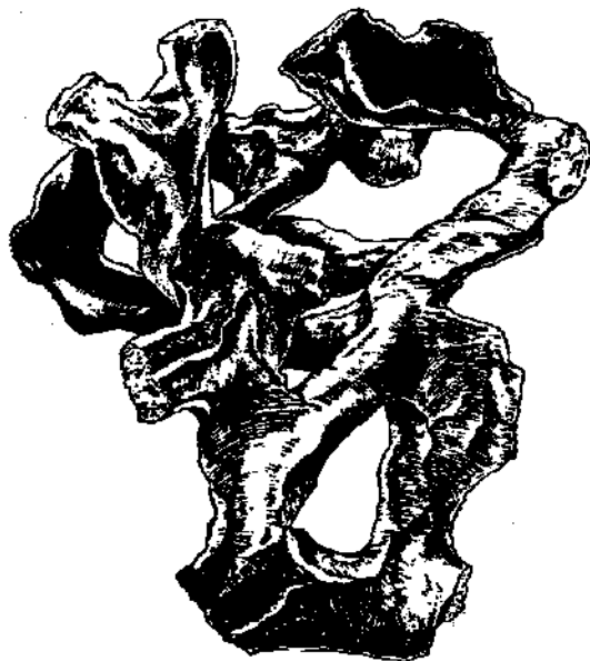
FIG. 2-24. Metallic cast of pore spaces in a consolidated sand. (Courtesy of Humble Oil & Refining Co.)
