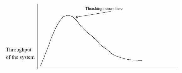
Page fault frequency Figure 4.11: Thrashing on numerous page fault.
