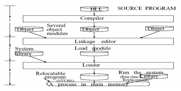
Figure 4.2: Linking and loading.
