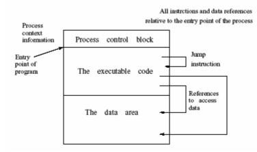
Figure 4.1: The relocation concept.
