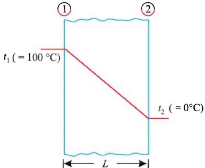
$$\begin{aligned} Q &= -kA \frac{dt}{dx} \\ q &= \frac{Q}{A} = -k \cdot \frac{(t_2 - t_1)}{L} \\ &= -387.6 \times \frac{(0 - 100)}{0.25} \\ &= \mathbf{1.55 \times 10^5 \text{ W/m}^2} \end{aligned}$$
