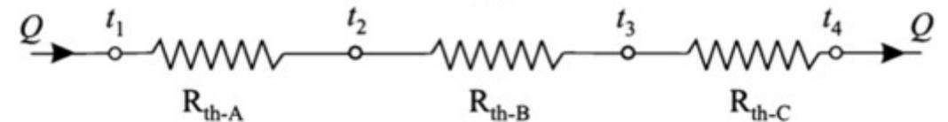
$$R_{th,A} = \frac{L_A}{k_A \cdot A}, \quad R_{th,B} = \frac{L_B}{k_B \cdot A}, \quad R_{th,C} = \frac{L_C}{k_C \cdot A}$$
