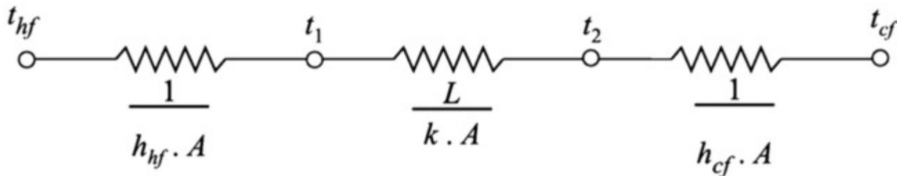
$$Q = h_{hf} A (t_{hf} - t_1)$$
