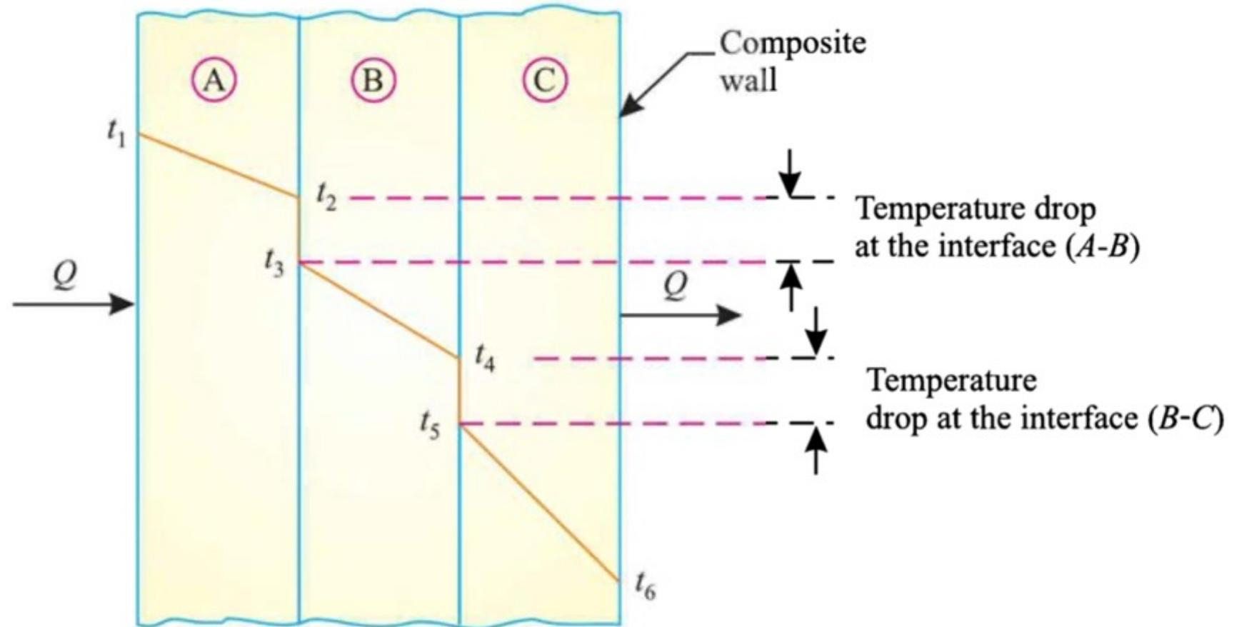
$$(R_{th-AB})_{cont} = \frac{(t_2 - t_3)}{Q/A}$$
