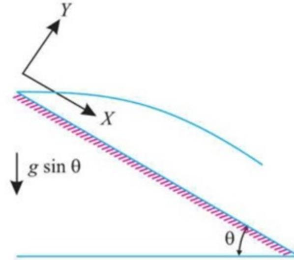
**Fig. 9.9.** Condensation on an inclined surface.
