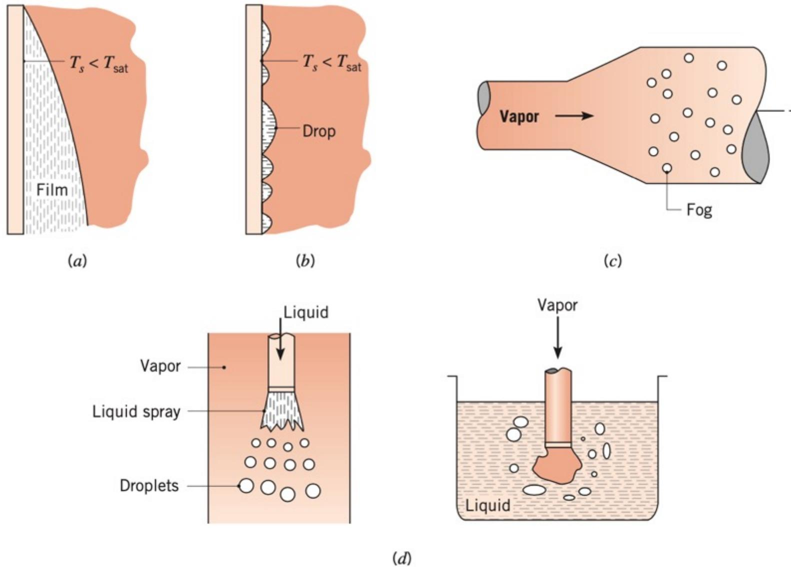
**FIGURE 10.9** Modes of condensation. (a) Film. (b) Dropwise condensation on a surface. (c) Homogeneous condensation or fog formation resulting from increased pressure due to expansion. (d) Direct contact condensation.
