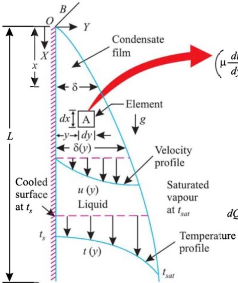
(a) Film growth, velocity and temperature profiles
