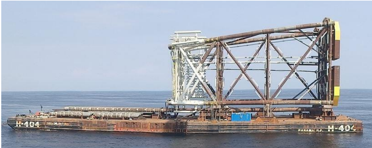
Gambar 1. Contoh Marine Operation: Transportasi Jacket [1]
