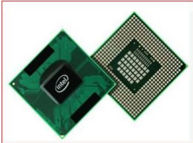
**Gambar 3.2 Chip Processor**
